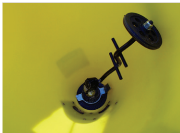
Our agitator is standard equipment and is useful when spreading powder type materials that tend to bridge.
