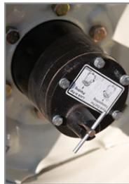
**LOCK OUT HUBS** - Disengages all drive components for transport reducing wear and tear.
