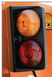
**SAFETY LIGHTS** - LED lights provide high visibility and safety during transport.
