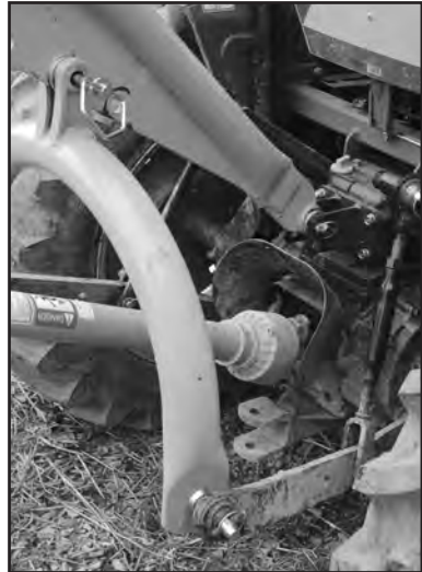
Having a Power Take Off (PTO) feature enables the tractor to drive rotary implements.
