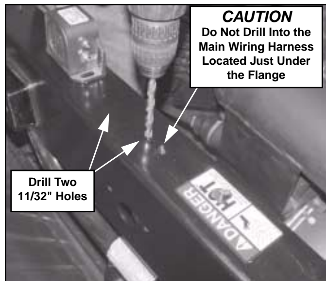
Drilling Mounting Holes Figure 10
