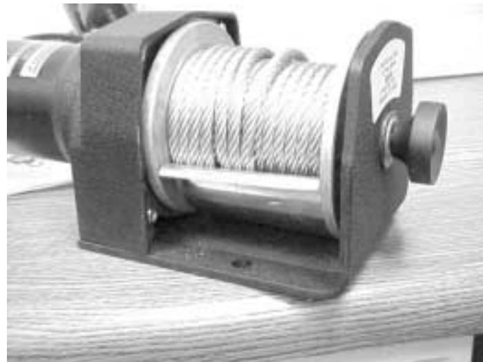
Keep in mind that maximum pulling capacity becomes less as more layers of cable are added. Working load of 2000 pounds is based on one layer of cable.
