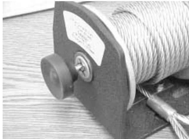
A Tension plate mounted on the winch reduces snarling and backlash while pulling the cable out.
